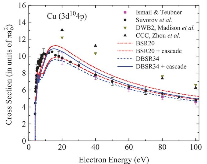
FIG. 3. (Color online) The same as Fig. 2 over an extended range of incident energies. The experimental data of Ismail and Teubner [9] and Suvorov *et al.* [2] are compared with predictions from nonrelativistic DWB2 [6], CCC [7], and BSR20 calculations, as well as the fully relativistic DBSR34 model. The effect of cascading is also illustrated in the (D)BSR curves.
