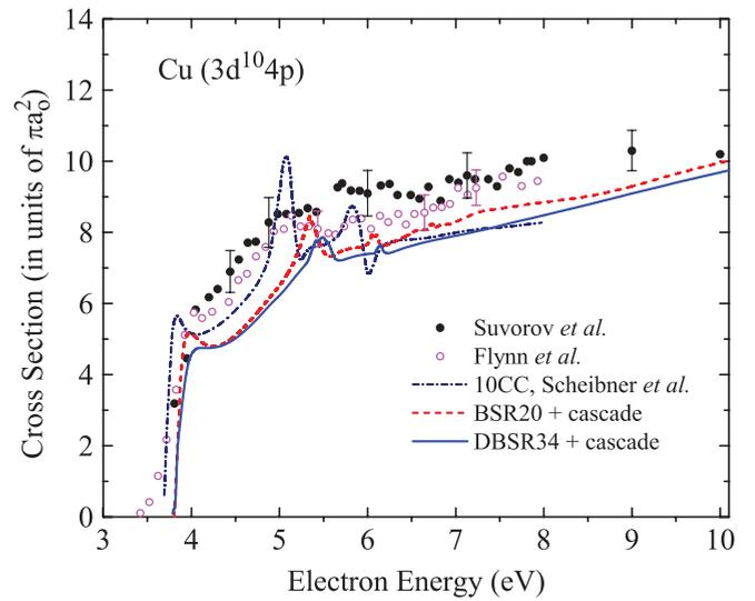
FIG. 2. (Color online) Excitation function of the  $(3d^{10}4p)^2P$  state in copper. The experimental data of Flynn *et al.* [17] and Suvorov *et al.* [2] are compared with predictions from a nonrelativistic standard 10-state close-coupling calculation [18], a nonrelativistic 20-state BSR (BSR20) model, and a fully relativistic 34-state (DBSR34) approach. The (D)BSR results include cascade contributions.
