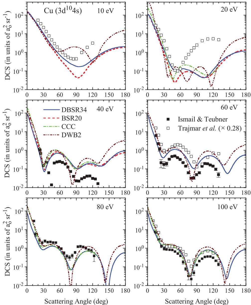
FIG. 4. (Color online) DCS for elastic electron scattering from copper at energies ranging between 10 and 100 eV. The nonrelativistic DWB2 [6], CCC [7], and BSR20 predictions, as well as the fully relativistic DBSR34 results, are compared with the experimental data of Trajmar *et al.* [8] and Ismail and Teubner [9]. The former data were multiplied by a factor of 0.28.
