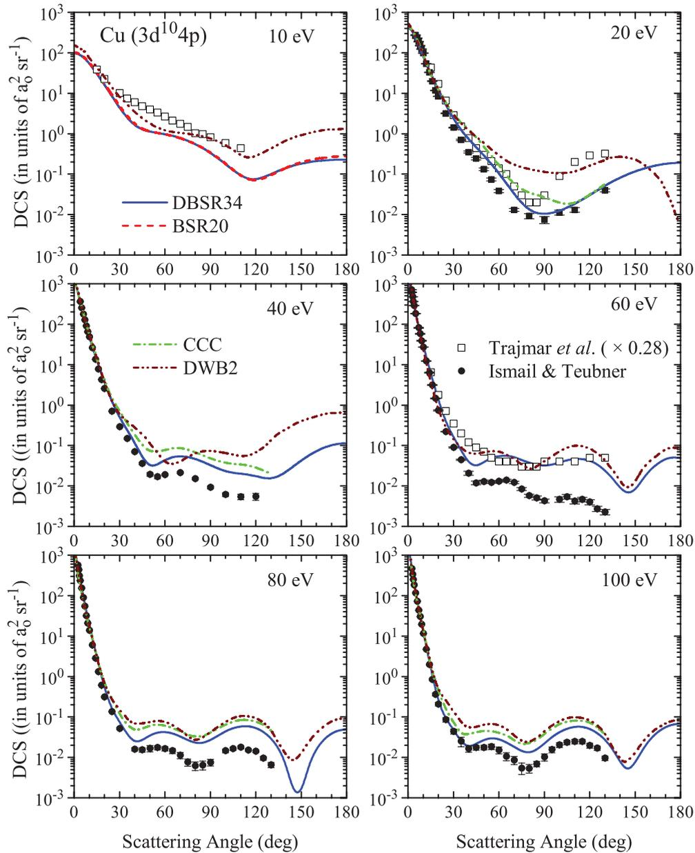
FIG. 5. (Color online) The same as Fig. 4 for electron-impact excitation of the  $(3d^{10}4p)^2P$  state in copper.
