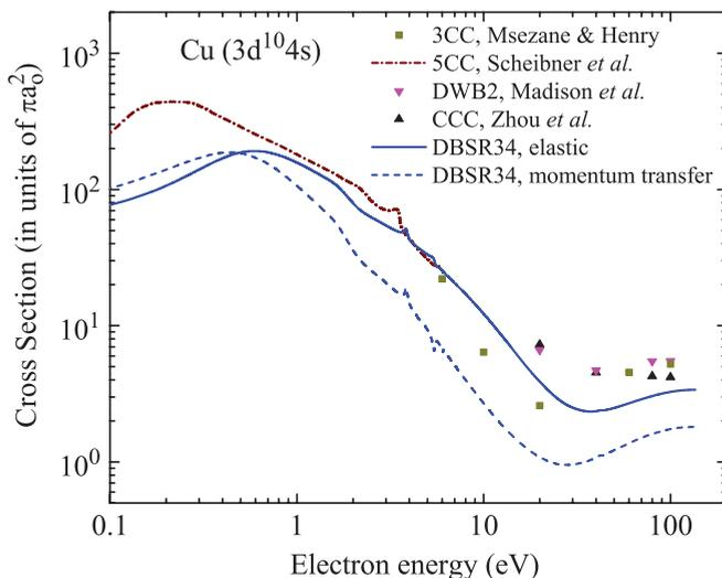
FIG. 1. (Color online) Angle-integrated elastic and momentum-transfer cross section for electron scattering from copper in its  $(3d^{10}4s)^2S$  ground state. The results for the elastic cross section from various nonrelativistic calculations, including a second-order distorted-wave (DWB2) model [6] as well as three-state (3CC) [14], five-state (5CC) [15], and CCC [7] models, are compared with the present DBSR34 predictions.
