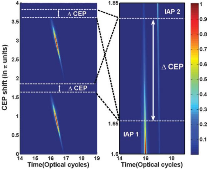
FIG. 4. (Color online) Left: Temporal intensity profile of the IAP as a function of CEP (from 0 to  $4\pi$ ), showing a  $2\pi$  periodic structure. Right: The enlargement of the part obtained with CEP from  $1.6\pi$  to  $1.85\pi$ . The laser parameters and the silica plate thickness are the same as those in Fig. 1.
