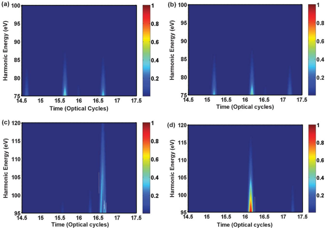
FIG. 2. (Color online) Diagrams of the time-frequency distribution for harmonic emission produced by the (a,b) chirp-free and (c,d) chirped driving laser field. The CEP values are (a,c)  $\delta_{\text{CEP}} = 0.4\pi$  and (b,d)  $\delta_{\text{CEP}} = 1.3\pi$ , respectively. The laser parameters and the silica plate thickness are the same as those in Fig. 1.
