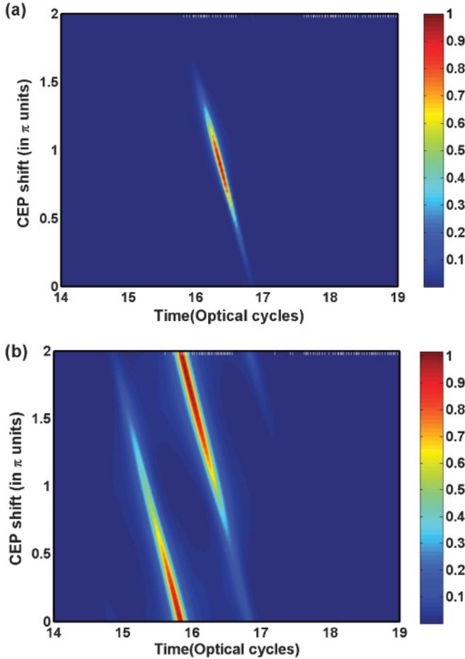
FIG. 1. (Color online) Temporal intensity profiles of the harmonic emission as functions of CEP, for the harmonic emission (a) in the range of 97–117 eV generated in the chirped laser field and (b) in the range of 77–97 eV generated in the chirp-free laser field. The time delay between the two-color pulses as 5.79 fs and the thickness of the fused silica plate is 1.0 mm.
