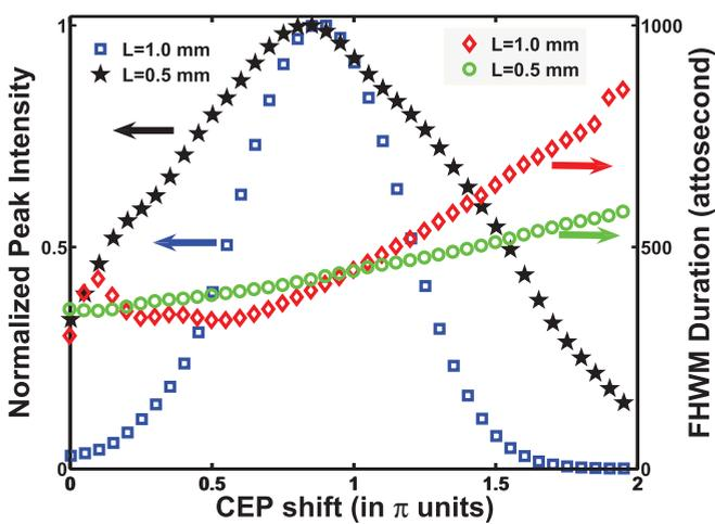
FIG. 3. (Color online) The intensity and pulse width of IAP as functions of CEP when the thickness of the fused silica plate is 0.5 mm (stars and open circles) and 1.0 mm (squares and open diamonds), respectively. The IAP corresponds to the harmonic emission from 97 to 117 eV produced in the chirped laser field. Note that the time delay between the two-color pulses is 4.98 fs for  $L = 0.5$  mm and 5.79 fs for  $L = 1.0$  mm, respectively.
