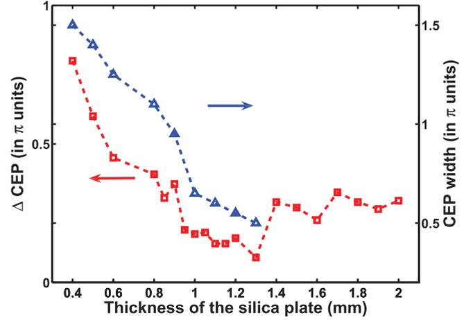
FIG. 5. (Color online)  $\Delta\text{CEP}$  and CEP width as functions of the thickness of the silica plate, calculated for the IAP corresponding to the harmonic emission from 97 to 117 eV produced in the chirped laser field. Note that the time delay between the two pulses is optimized for each value of the silica plate thickness.
