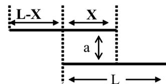
FIG. 1. Two square  $L \times L$  parallel perfectly conducting plates with an overlapping area  $L \times X$ , separated by a distance  $a$ . Only lateral motion is permitted.
