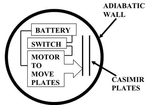
FIG. 3. Schematic showing apparatus described in gedanken experiment 3, consisting of a motor-generator to alter the spacing between two parallel plates, a battery to power the motor, and a timer switch, all surrounded by a wall impervious to thermal energy and matter.
