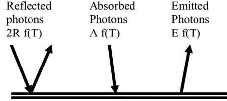
FIG. 2. Schematic of the momentum transfer from electromagnetic radiation to a sail made of different materials on the top and bottom.
