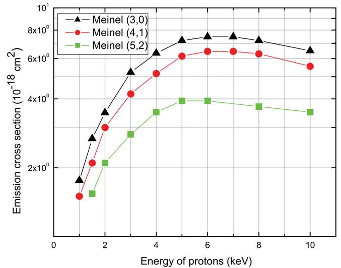
FIG. 4. (Color online) Dependence of excitation cross sections for the Meinel (3,0), (4,0), and (5,2) band systems on the proton energy for  $p$ - $N_2$  collisions.
