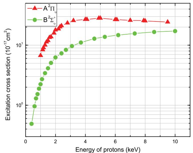
FIG. 5. (Color online) Dependence of the manifold excitation cross section for the  $A^2\Pi_u$  and  $B^2\Sigma_u^+$  states on the proton energy for  $p$ - $N_2$  collisions.
