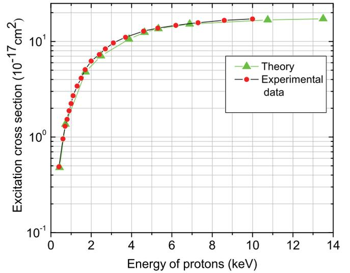
FIG. 6. (Color online) Dependence of the excitation cross section for the first negative band system on the proton energy for  $p$ - $N_2$  collisions.
