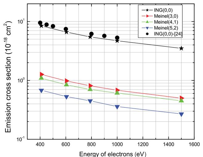
FIG. 3. (Color online) Dependence of the excitation cross sections for the first negative (0,0) and Meinel (3,0), (4,0), and (5,2) band systems on the electron energy for the  $e-N_2$  collision.
