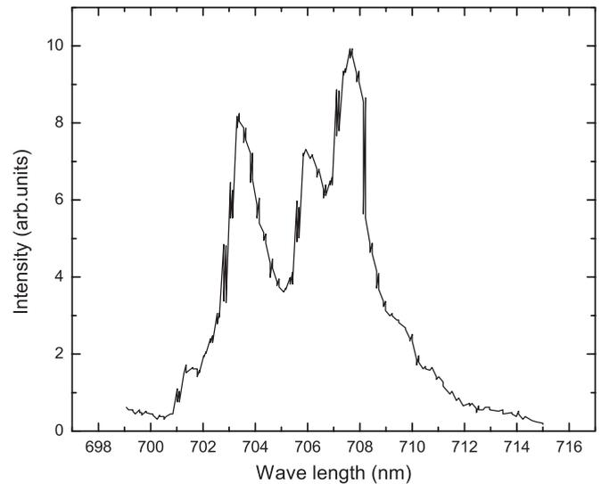
FIG. 2. Experimental spectrum of the  $N_2^+$  Meinel (4,1) band for an electron energy of 400 eV.
