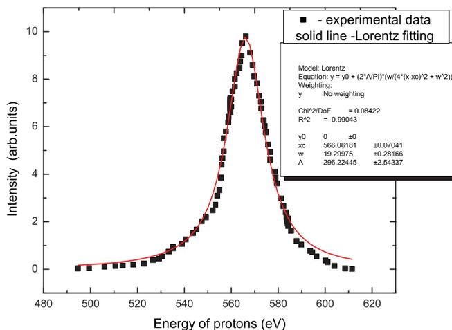
FIG. 1. (Color online) Dispersion of the proton energy for the acceleration potential of 600 V.
