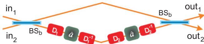
FIG. 2. (Color online) Schematic representation of the two-mode controlled PHASE gate. \text{BS}_b stands for a balanced beam splitter and D_{1,2} represent displacements by \gamma_{1,2}/\sqrt{2} . Numbers 1 and 2 distinguish the two participating modes, while labels “in” and “out” describe the input and output states of the gate.
