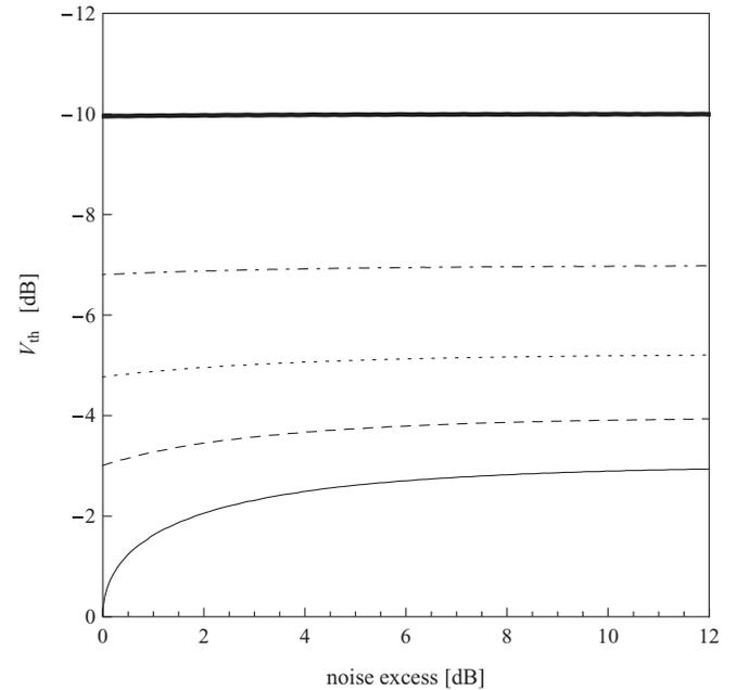
FIG. 12. Threshold squeezed variance  $V_{\text{th}}$  versus the noise excess for conditional teleportation of input state  $\eta|1\rangle\langle 1| + (1 - \eta)|0\rangle\langle 0|$  for  $\eta = 1$  (solid curve),  $\eta = 0.9$  (dashed curve),  $\eta = 0.8$  (dotted curve),  $\eta = 0.7$  (dash-dotted curve), and  $\eta = 0.6$  (thick solid curve), where we accept only the result  $\beta = (\bar{x}_u + i\bar{p}_v)/\sqrt{2} = 0$ .
