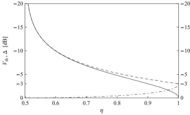
FIG. 6. Threshold squeezed variances  $V_{\text{th}}^{(G)}$  (solid curve) and  $V_{\text{th}}^{(1)}$  (dashed curve) and their difference,  $\Delta = V_{\text{th}}^{(1)} - V_{\text{th}}^{(G)}$  (dash-dotted curve), versus the probability  $\eta$ . See text for details.
