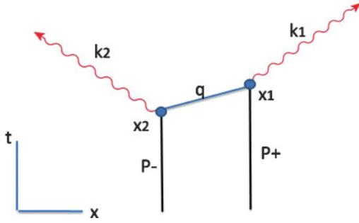
FIG. 1. (Color online) A two-photon Feynman diagram. An electron,  $p_-$ , emits a photon,  $k_2$ , while scattering to a virtual state,  $q$ . It then annihilates with a positron,  $p_+$ , while creating a second photon,  $k_1$ .
