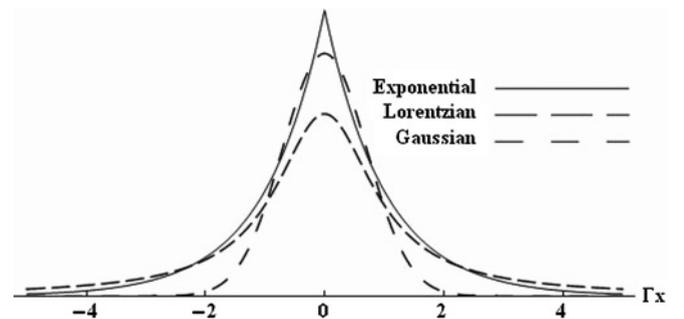
FIG. 3. Comparison of exponential of the absolute value  $(2\Gamma)^{-1} \exp(-\Gamma|x|)$  with a Lorentzian,  $(\pi\Gamma^2)^{-1}(x^2 + \Gamma^2)^{-1}$  and a Gaussian  $(\Gamma\pi)^{-3/2} \exp(-\Gamma^2 x^2)$ .
