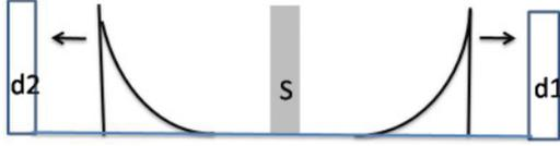
FIG. 2. (Color online) Irby experiment. A positron is created in the source  $S$  and the time difference between annihilation photons arriving at detectors  $d1$  and  $d2$  is measured.
