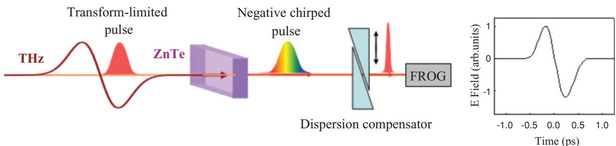
FIG. 2. (Color) (a) Schematic diagram of the experimental setup. (b) Measured THz wave form.
