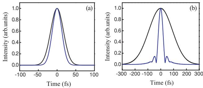
FIG. 1. (Color) Simulated pulse compression with a 40 fs (a) and 180 fs (b) probe pulse. The black and blue lines show input pulse and compressed pulse, respectively. The compression ratio is 1.3 and 4.5 for the 40 and 180 fs input pulse.
