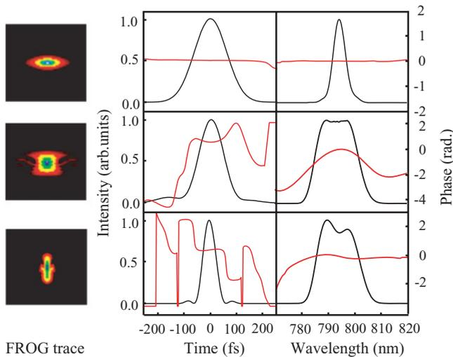
FIG. 3. (Color) Experimental results of FROG measurements. Column 1, measured SHG FROG traces. Columns 2 and 3, retrieved intensity (black) and phase (red) in time and frequency domains. The top and middle rows show the probe pulses in the absence and the presence of THz pulse. The bottom row shows the compressed or focused probe pulse.
