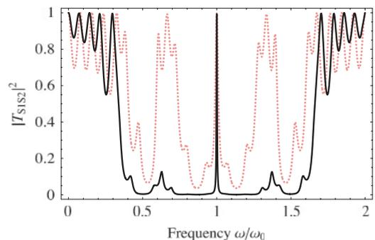
FIG. 6. (Color online) Transmission spectrum of the structure in Fig. 4(a) for  $n_A = 1.55, n_B = 2.3$  as in [15] (dotted line) and for increased  $n_B/n_A$  by setting  $n_A = 1$  (solid line).
