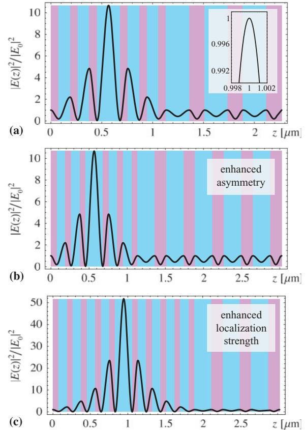
FIG. 5. (Color online) Electric field localization profile at the PTR frequency  $\omega = \omega_0$  (cf. inset) for the proposed structure design [Eq. (10)] for (a)  $k = m = 3$  as in Fig. 4; (b)  $k = 3, m = 5$  (enhanced asymmetry); and (c)  $k = 5, m = 3$  (enhanced localization strength).
