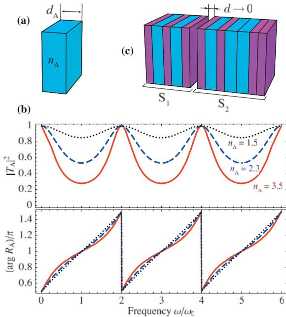
FIG. 2. (Color online) (a) A single layer and (b) its transmittance  $|T_A|^2$  and phase shift of the reflected wave  $\varphi_A$ , given by Eq. (1), for different values of  $n_A$  [ $d_A$  is chosen in accordance with Eq. (2)]; (c) an example of a composite  $S_1 S_2$  structure described by Eq. (3).
