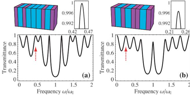
FIG. 1. (Color online) Example transmission spectra of (a) symmetric Cantor multilayer  $BABAAABAB$  and (b) nonsymmetric Fibonacci multilayer  $BABABBAB$ .  $A$  and  $B$  correspond to single layers with  $n_A = 1.55$ ,  $d_A = 76$  nm, and  $n_B = 2.3$ ,  $d_B = 113$  nm, so that  $n_A d_A = n_B d_B = \pi c / 2\omega_0 = \lambda_0 / 4$  for  $\lambda_0 = 700$  nm as in [15]. The insets show an enlarged view of the transmission peaks marked by arrows.
