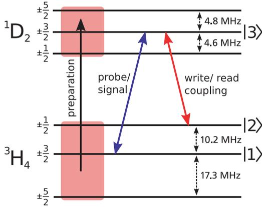
FIG. 1. (Color online) Coupling scheme in Pr:YSO.
