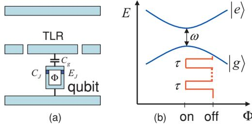
FIG. 4. (Color online) (a) Schematic diagram of the circuit QED system of a transmission line resonator (TLR) coupled with a charge qubit, which is controlled through an external magnetic flux  $\Phi$  and a gate voltage  $V$ . (b) The energy levels of the charge qubit versus the magnetic flux  $\Phi$ , the working status of the qubit is controlled by the magnetic flux “pulse series”. By tuning the magnetic flux  $\Phi$ , we can switch on or off the coupling between the TLR and the charge qubit.
