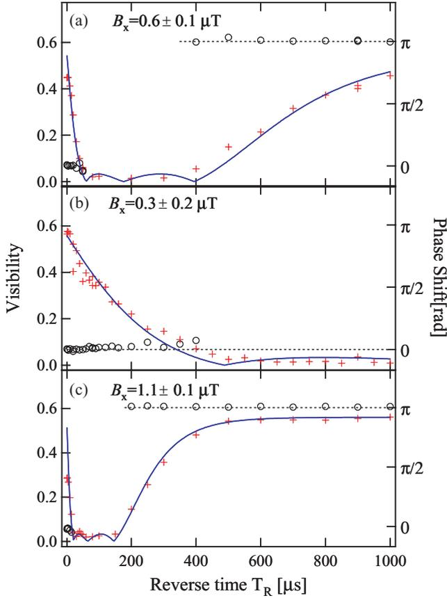
FIG. 3. (Color online) Visibility (+) and phase shift (o) of fringes as a function of reverse time  $T_R$ , together with calculated curves of visibility using Majorana transitions.  $B_z = 5.0 \mu\text{T}$ . The fitted values of  $B_x$  are 0.95 for (a), 0.32 for (b), and 1.6  $\mu\text{T}$  for (c).
