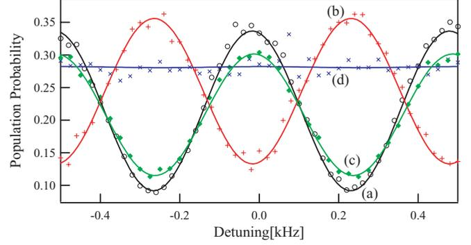
FIG. 2. (Color online) Observed Ramsey fringes with (a) constant magnetic field, (b) reverse magnetic field of  $f_{\text{rot}} = 2.7$  kHz (adiabatic regime), (c)  $f_{\text{rot}} = 2.7$  MHz (nonadiabatic regime), and (d)  $f_{\text{rot}} = 8.8$  kHz (intermediate region).
