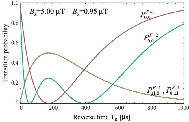
FIG. 4. (Color online) Majorana transition probabilities  $P_{m,m'}^F$  from  $m$  to  $m'$  in the  $F$  state, which are related to the population probabilities in the  $F = 2$ ,  $m_F = 0$  state, for various reverse times under the conditions of  $B_x = 0.95 \mu\text{T}$  and  $B_z = 5.00 \mu\text{T}$ .
