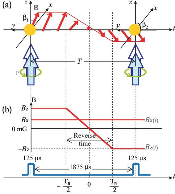
FIG. 1. (Color online) (a) Schematic of phase measurement of the Ramsey atom interferometer. Two  $\sigma^+ - \sigma^+$  polarized two-photon Raman pulses separated by  $T$  propagate in the  $z$  direction and interact with a cold ensemble of sodium atoms. The direction of the magnetic field rotates around the  $y$  axis. (b) Timing diagram of magnetic fields of  $B_x(t) = B_x$  and  $B_z(t)$  and two Raman pulses.  $B_z(t)$  reverses from  $B_z$  to  $-B_z$  with reverse time of  $T_R < T$ .
