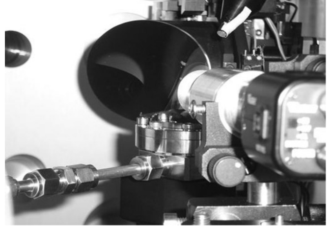
FIG. 4. Picture from inside of the laser interaction area of the intense laser with the He gas jet. The off-axis mirror which was used to focus laser beams with the waist of 1.38 \text{ cm}^2 at a 100\text{-}\mu\text{m}^2 spot at the tip of the nozzle is shown.
