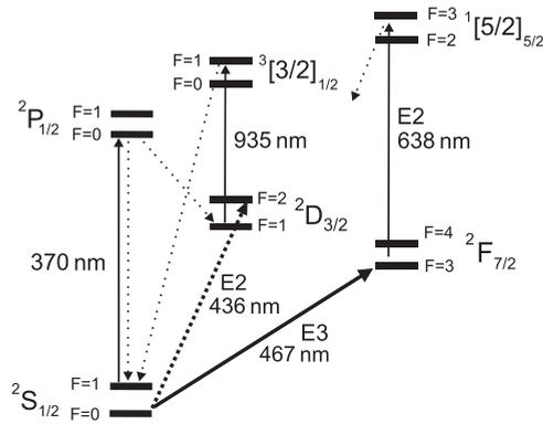
FIG. 1. Simplified level system of  $^{171}\text{Yb}^+$  showing the employed laser cooling (370 nm) and repumping excitation (935 nm, 638 nm) and major spontaneous decay paths (dotted lines). Optical clocks can use the dipole-forbidden 436- and 467-nm transitions from the ground state as reference transitions.
