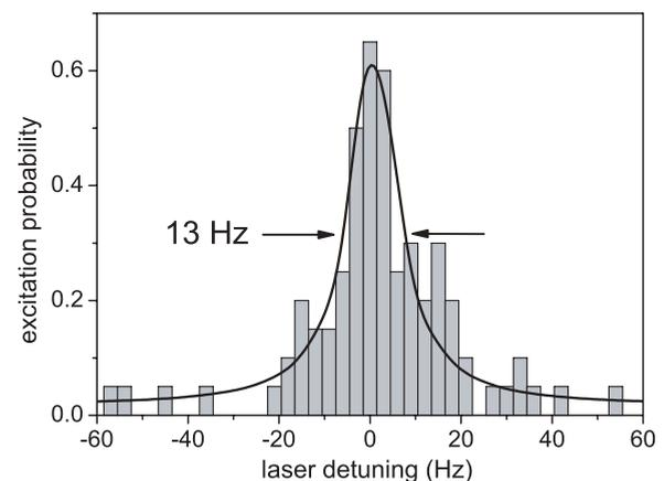
FIG. 5. Observed excitation spectrum of the  $^2S_{1/2} (F=0) \rightarrow ^2F_{7/2} (F=3, m_F=0)$  transition of a trapped  $^{171}\text{Yb}^+$  ion. The superimposed line is a least-squares Lorentzian fit.
