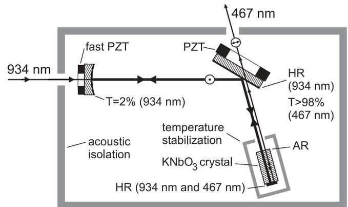
FIG. 3. Setup for frequency doubling of 934-nm radiation, showing the beam geometry and polarization orientations in the semimonolithic enhancement cavity. T, transmissivity; HR (AR), high-reflectivity (antireflection) coating.
