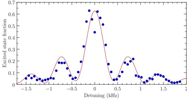
FIG. 5. (Color online) Excitation fraction as a function of probe laser detuning for a probe time of 1.7 ms. The solid curve is a fit of Eq. (18) with the temperature as the only free parameter fixing  $\Delta\theta$  at 10 mrad. The fit gives  $T_z=T_r=(2.1\pm 0.2)$   $\mu\text{K}$  consistent with the sideband method and time-of-flight expansion.
