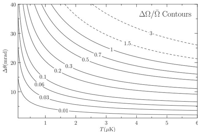
FIG. 6. Contour plot of the relative spread in Rabi frequency  $\Delta\Omega/\bar{\Omega}$  as a function of misalignment angle  $\Delta\theta$  and temperature  $T_z=T_r=T$ . The dashed contour lines indicate points where the mean Rabi frequency becomes smaller than the rms spread made possible by the negative values of the Laguerre polynomials in Eq. (14) for large radial quantum numbers. The experimentally relevant range is  $\Delta\Omega/\bar{\Omega}=0.05-0.4$ .
