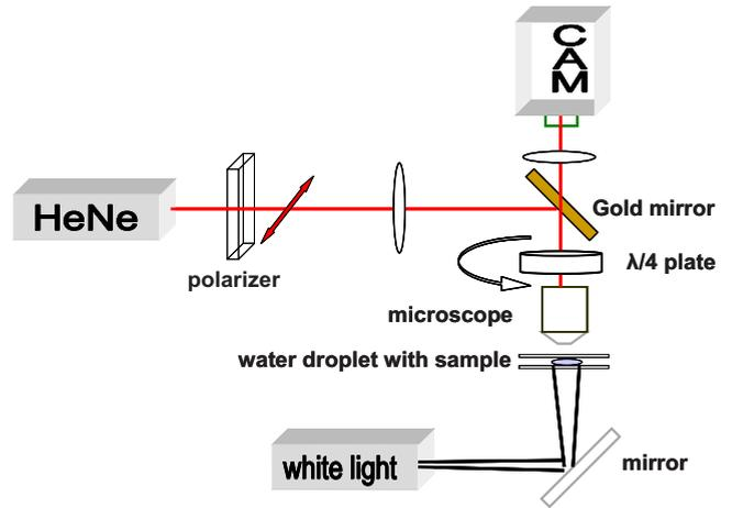
FIG. 6. (Color online) Birefringent platelets were held in optical tweezers and filmed with a video camera. The tweezing light from a HeNe laser was polarized with a polarizer and a rotatable quarter wave plate. The beam was focused via a gold mirror and the high aperture microscope objective onto the object slide with the sample suspension of the microcrystals in water.
