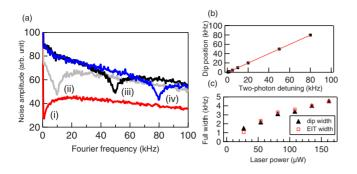
FIG. 2. (Color online) (a) Measured noise spectra of total transmitted power for hyperfine EIT. Two-photon detunings of (i) 1, (ii) 10, (iii) 50, and (iv) 80 kHz. (b) Dip center frequencies vs twophoton detuning (symbols); line represents *dip center=detuning*. (c) Widths of dips and EIT resonances are equal at all input laser powers. (Two-photon detuning=50 kHz.) Laser power  $\approx$ 170  $\mu$ W for plots (a) and (b). 0.85 mm beam size and 2 Torr Ne buffer gas for (a)–(c).
