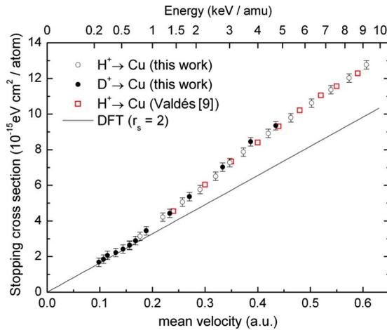
FIG. 2. (Color online) Stopping cross section for hydrogen ions in Cu, as a function of the mean projectile velocity (with the equivalent energy shown in the upper scale). Open circles show proton data, full circles correspond to deuterons. Open squares are previous data of Valdés *et al.* [9]. The high energy value of this data was used as reference stopping power in this work. Solid line corresponds to a DFT calculation for a free-electron gas with  $r_s = 2$  a.u.
