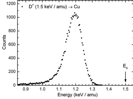
FIG. 1. Energy spectrum of 1.5 keV/amu deuterons transmitted through a 157 Å Cu foil.
