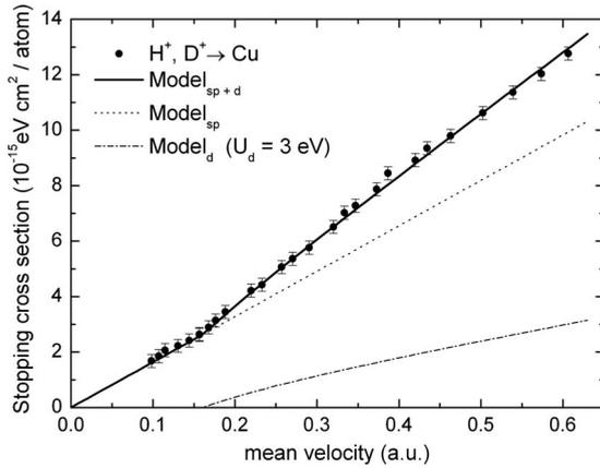
FIG. 4. Stopping cross section for protons and deuterons in copper. Full circles: present experimental results. Curves: solid line, theory total result; dotted line, free electron contribution; dash-dotted line, nearly-free-electron contribution. The minimum energy transfer of the  $d$  electrons in this calculation is  $U_d=3$  eV.
