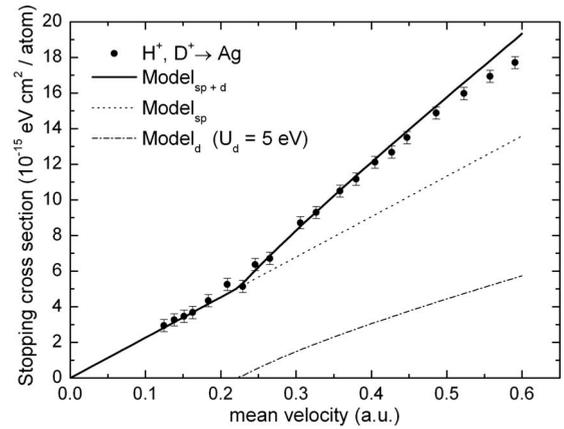
FIG. 5. Stopping cross section for protons and deuterons in silver. Full circles: present experimental results. Curves: solid line, theory total result; dotted line, free-electron contribution; dash-dotted line, nearly-free-electron contribution. The minimum energy transfer of the  $d$  electrons in this calculation is  $U_d=5$  eV.
