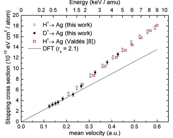
FIG. 3. (Color online) Stopping cross section for hydrogen ions in Ag, as a function of the mean projectile velocity (with the equivalent energy shown in the upper scale). Open circles show proton data, full circles correspond to deuterons. Open squares are previous data of Valdés *et al.* [8]. The high energy value of this data was used as reference stopping power in this work. Solid line corresponds to a DFT calculation for a free-electron gas with  $r_s = 2.1$  a.u.
