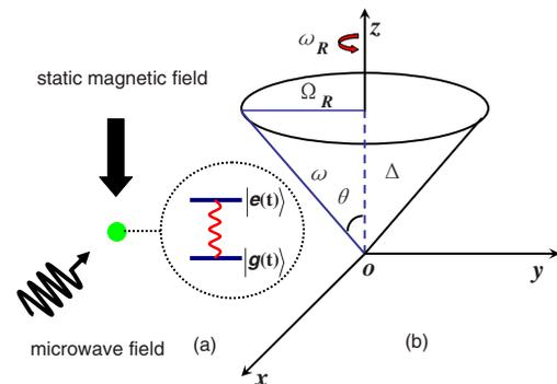
FIG. 1. (Color online) (a) Schematic of a TLS in a static magnetic field along with a microwave field. (b) Realized effective Hamiltonian rotating in the parametric space.
