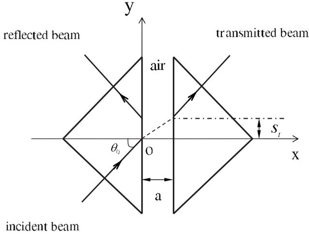
FIG. 1. Schematic diagram of the GH shift  $s_t$  in FTIR, where the width of air gap is  $a$ .
