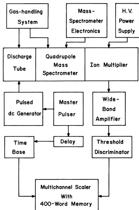
FIG. 1. Block diagram of measuring system.
