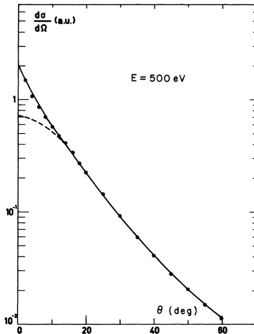
FIG. 2. Elastic scattering of electrons by helium at 500 eV. Solid curve represents the eikonal-Born-series theoretical results, while the dashed curve represents the "static-plus-exchange" calculation. Circles show the experimental results of Ref. 4.
