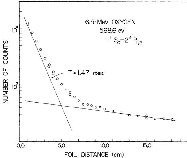
FIG. 2. Decay curve for the He-like  $1^1S_0(1s)^2-2^3P(1s)(2p)$  transition. The short-lived component has a 1.47-nsec lifetime and is identified with the decay of the  $2^3P_1$ .
