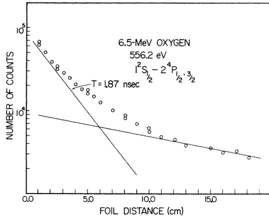
FIG. 4. Decay curve for the Li-like  $1^2S_{1/2}(1s)^2(2s)-2^4P(1s)(2s)(2p)$  transition. The short-lived component has a 1.87-nsec lifetime that is probably due to the  $2^4P_{3/2}$  transition.
