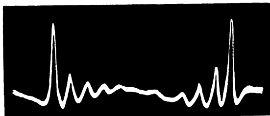
FIG. 4. Zeeman pattern of the \nu_+(5) fine-structure transition in ^{18}\text{O}_2 . The increasing height of the outer components is due to their greater sensitivity to Zeeman modulation.
