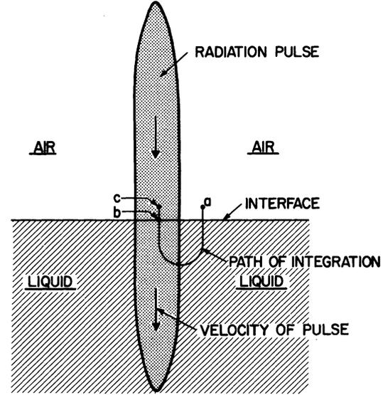
FIG. 4. Radiation pulse passing an air-liquid interface. A reflected pulse is actually present but is not illustrated.
