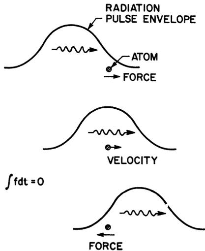
FIG. 1. A plane-wave pulse passing through a gas of atoms. The force on a representative gas atom is illustrated.
