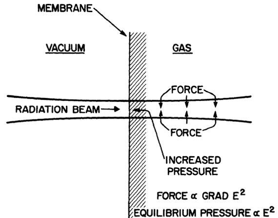
FIG. 2. A beam of radiation continuously passing a vacuum-gas interface.
