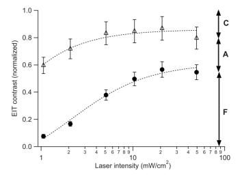
FIG. 3. Measured EIT floor ( $\mathbf{F}$ , circles) and peak transmission ( $\mathbf{F}$ + $\mathbf{A}$ , triangles) level vs total laser intensity for experimental conditions described in the text. Uncertainties in the measured contrasts in this figure are predominantly systematic. Dotted curves are fits of a four-level model to the data with good agreement between fit parameters and experimental conditions (see text).
