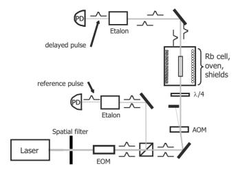
FIG. 2. Schematic of the apparatus used for our EIT and slowlight measurements. An electro-optic modulator (EOM) frequency modulates the laser light to generate signal and reference field sidebands, while an acousto-optic modulator (AOM) regulates the light intensity. Reference and output signal fields are sent into photodetectors (PD) for EIT line shape and slow-light delay measurements. See text for details.
