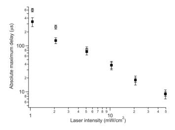
FIG. 4. Measured slow-light delays (solid squares) and predictions (hollow squares) based on accessible EIT line-shape parameters. Good agreement is shown over a large range of pulse delays and laser intensities.
