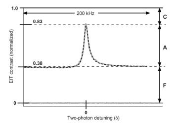
FIG. 1. Intensity spectrum with normalized contrast and background levels. Solid gray line is the data while the dashed dark line is a fit to a skew-Lorentzian. F: signal intensity above background away from EIT resonance (the "floor"); A: amplitude of EIT peak; C: difference between EIT peak and 100% transmission (the "ceiling"). Parameters are normalized so that F+A+C=1. (For data shown here, T=40 °C, in 25 torr N<sub>2</sub> buffer gas, and total laser power  $\approx 490 \ \mu W.$ )
