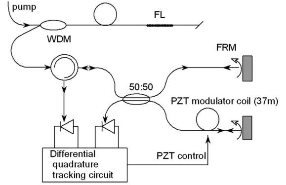
FIG. 1. The experimental setup used to measure frequency noise.
