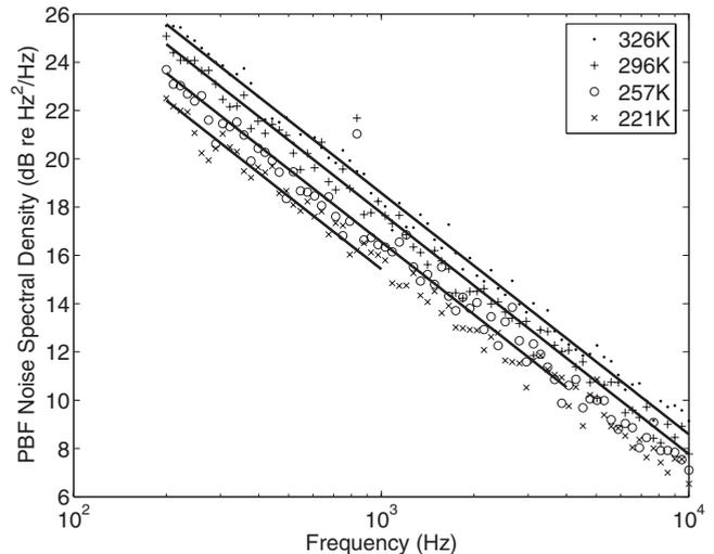
FIG. 6. One-sided power spectral density of the polarization-beat-frequency noise vs temperature.
