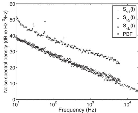
FIG. 5. Polarization resolved (one-sided) frequency noise spectra of a dual-polarization DFB fiber laser, labeled  $S_{v_1}$  and  $S_{v_2}$  for the respective polarization modes. Also shown is the difference between the two spectra ( $S_{v_b}$ ) and the polarization-beat-frequency noise measured directly (PBF).
