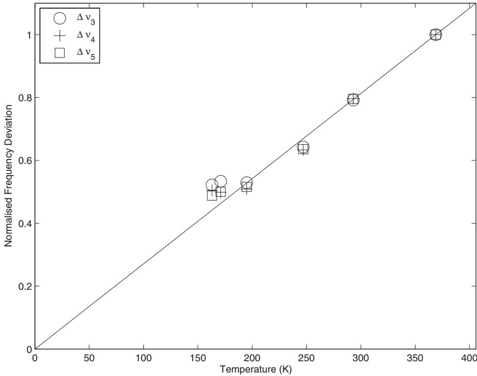
FIG. 3. Estimated rms laser frequency deviation versus temperature (normalized to unity at 369 K):  $\Delta\nu_5$  (“□”) includes noise contributions up to  $10^5$  Hz;  $\Delta\nu_4$  (“+”) includes contributions up to  $10^4$  Hz;  $\Delta\nu_3$  (“○”) includes contributions up to  $10^3$  Hz. Noise contributions below 60 Hz and between 250 and 350 Hz have been excluded.
