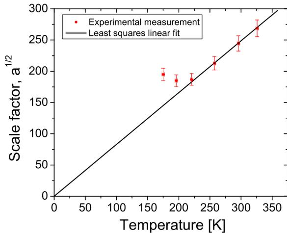
FIG. 7. (Color online) Scale factor  $a^{1/2}$  obtained from a nonlinear curve fit of polarization-beat-frequency noise vs temperature.
