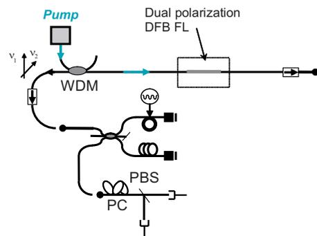
FIG. 4. (Color online) Experimental setup for measuring the polarization resolved frequency noise and temperature dependence of the polarization-beat frequency in a dual-polarization DFB fiber laser
