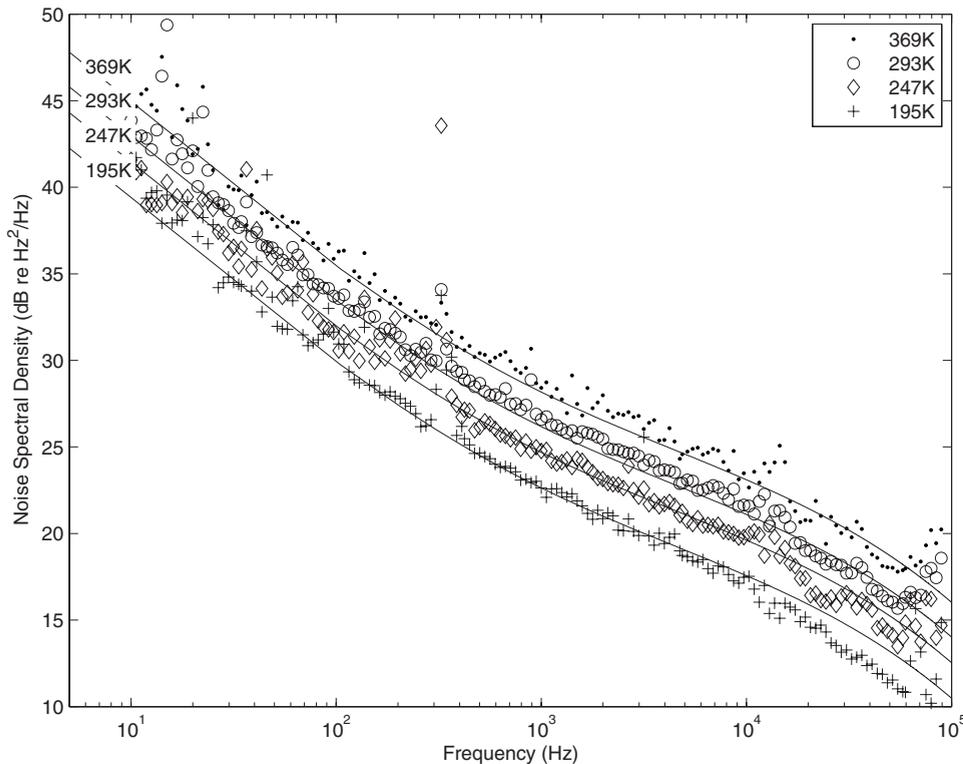
FIG. 2. Experimental one-sided DFB FL frequency noise  $[2S_{\nu}(f)]$  data measured at 369 K (“•”), 293 K (“○”), 247 K (“◇”) and 195K (“+”). Corresponding theoretical curves are shown as solid lines.
