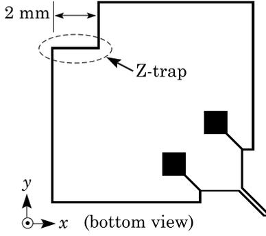
FIG. 1. Chip pattern of the superconductive strip.
