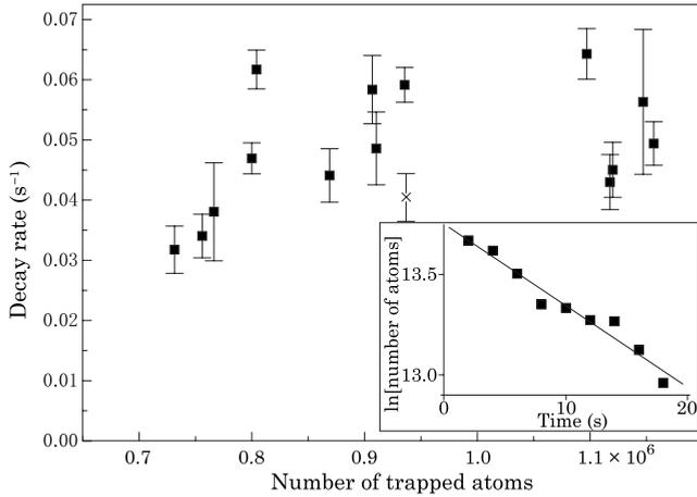
FIG. 3. Distribution of the decay rate as a function of the initial number of trapped atoms. The error bars show the errors of the individual decay rate measurements. All the data were obtained over a period of two months. The inset shows an example of the decay curve of the trapped atoms. These data correspond to the data points indicated by “x.”
