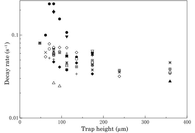
FIG. 4. Distribution of the measured decay rate of a trapped atomic cloud as a function of the trap height. Different symbols indicate data obtained on different dates. Clearly the distribution of data obtained on the same day is much smaller than the distribution of all the data. The error of each point is approximately  $\pm 10\%$  of the measured value.
