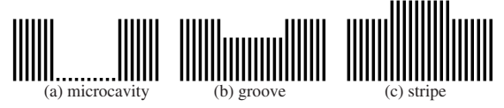
FIG. 1. Distribution of nanoparticles density in (a) RABG microcavity \gamma(\zeta)=0 , (b) RABG wide groove defect \gamma(\zeta)<1 , and (c) RABG wide stripe defect \gamma(\zeta)>1 .
