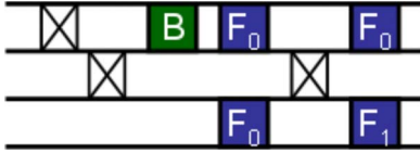
FIG. 2. (Color online) Quantum circuit that reproduces all the dynamical properties of the quantum Ising Hamiltonian in a external magnetic field with four spins. Some initial and final reordering gates can be sparsed in an experimental realization.
