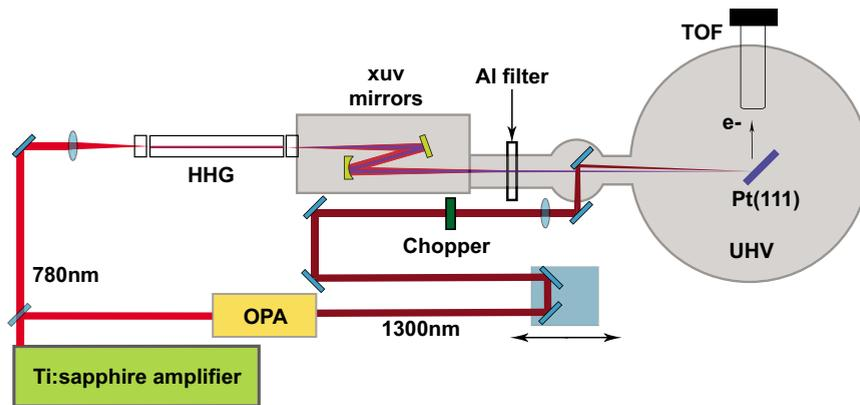
FIG. 1. (Color online) Experimental setup for observing the laser-assisted photoelectric effect from a Pt surface.
