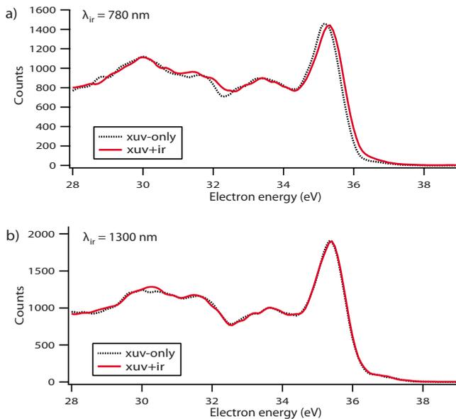
FIG. 4. (Color online) Comparison of space-charge effects around the Fermi edge at  $-100$  fs time delay between the xuv and ir pulses. For 780 nm pulses, the large number of low energy photoelectrons generated through ATP causes a shift of the entire photoemission spectrum around the Fermi edge. This effect is greatly suppressed with 1300 nm pulses, because of the smaller number of ATP photoelectrons.
