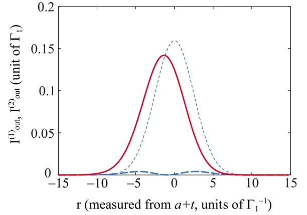
FIG. 3. (Color online) Intensity profiles of the one-photon output (dashed line) and the two-photon output (solid line). The input photon profile (thin dotted line) is also plotted for reference. The parameters are chosen as  $\Gamma_1 = \Gamma_2 = \Gamma_3$  and  $d = 5/\Gamma_1$ . Under this condition, the down-conversion probability  $P_2$  reaches 96.4%.
