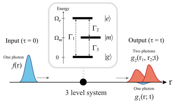
FIG. 1. (Color online) Schematic illustration of the situation considered in this study. A parent photon resonant to the  $|g\rangle \rightarrow |e\rangle$  transition is input into a three-level atom and is down-converted into two daughter photons with some probability. Under certain conditions, the parent photon can be down-converted with unit efficiency.
