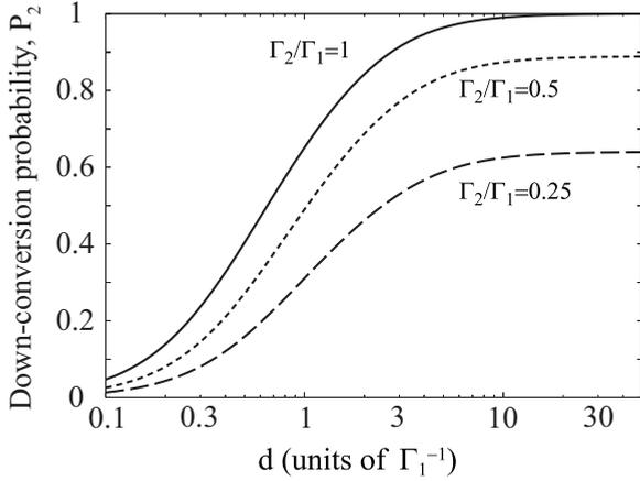
FIG. 2. Down-conversion probability  $P_2$  as a function of the coherence length  $d$  of the input photon.  $\Gamma_2/\Gamma_1$  is set at 1 (solid line), 0.5 (dotted line), and 0.25 (dashed line).
