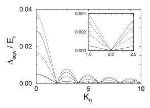
FIG. 2. Width  $\Delta_{\text{sqw}}$  of the lowest quasienergy band of an optical cosine lattice under square-wave driving as function of the dimensionless amplitude (29), for  $V_0/E_r$ =2 (dots), 3 (long dashes), 5 (short dashes), and 10 (full line). The inset illustrates that an exact band collapse occurs when  $K_0$  is a nonzero integer multiple of 2.
