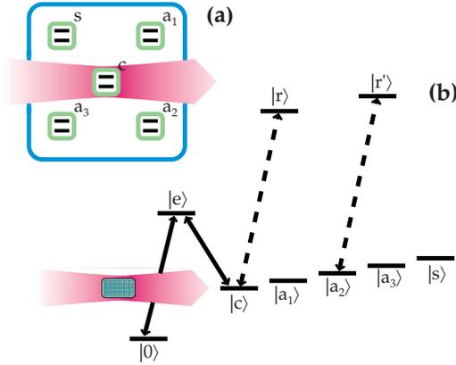
FIG. 2. (Color online) (a) A five-qubit register consisting of a communication qubit ( $c$ ), a storage qubit ( $s$ ), and three auxiliary qubits ( $a_{1,2,3}$ ) [28]. (b) The collective encoding implementation, with a collective internal state transition interacting with the field mode, and long lived and Rydberg internal states used for encoding and coupling of the five qubits.
