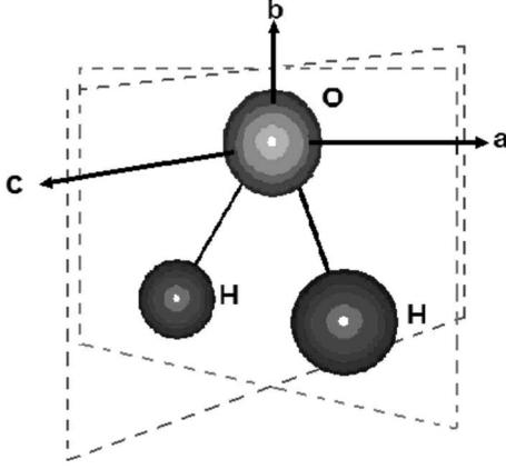
FIG. 1. The water molecule geometry. The axes are the principal axes of the molecule,  $a$ ,  $b$ , and  $c$  ( $a$  and  $b$  are in the molecular plane, and  $c$  is perpendicular to it). The principal moments of inertia are  $I_a=1.025 \times 10^{-47}$  kg m<sup>2</sup>,  $I_b=1.921 \times 10^{-47}$  kg m<sup>2</sup>, and  $I_c=2.946 \times 10^{-47}$  kg m<sup>2</sup> (note that  $I_c=I_a+I_b$  according to [9]).
