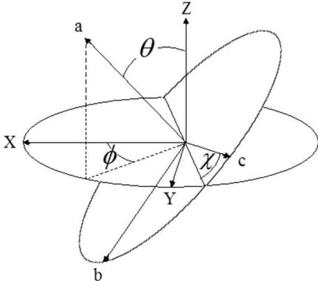
FIG. 2. The coordinate system. ( $X, Y, Z$ ) are the space fixed laboratory axes, ( $a, b, c$ ) are the body fixed principal axes, and ( $\theta, \phi, \chi$ ) are the Euler angles which define the body orientation in space with respect to the space fixed coordinates.
