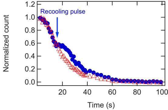
FIG. 6. (Color online) (●) Lattice population vs time showing the effect of a single 5-ms cooling pulse applied at  $t=15$  s. ( $\Delta$ ) Similar data without the cooling pulse applied.
