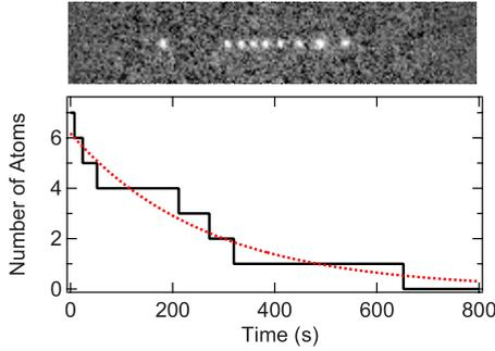
FIG. 2. (Color online) Top: continuously cooled array of  $^{87}\text{Rb}$  atoms trapped in a 1D optical lattice. Bottom: number of atoms vs time, starting from seven atoms initially loaded in the lattice. Dashed line is an exponential fit to the data.
