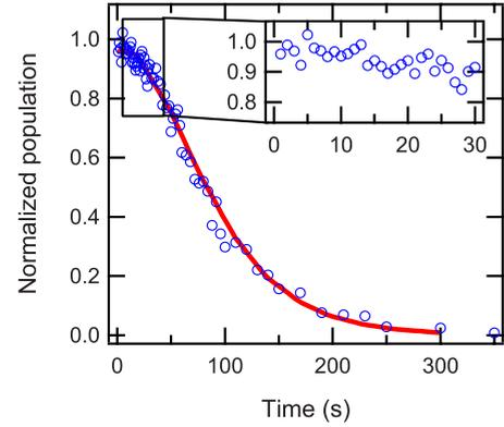
FIG. 3. (Color online) Atom population in the optical lattice vs time with no cooling. For each data point, the final population in the trap is normalized to the initial population. The asymptotic decay of the trap is exponential with a 62-s lifetime. Inset shows the trap population for the first 30 s. The solid line is a simulation including heating, as discussed in the text.
