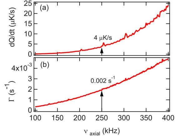
FIG. 5. (Color online) (a) Heating rate due to fluctuations in the axial trap position. (b) Heating time constant due to intensity fluctuations.
