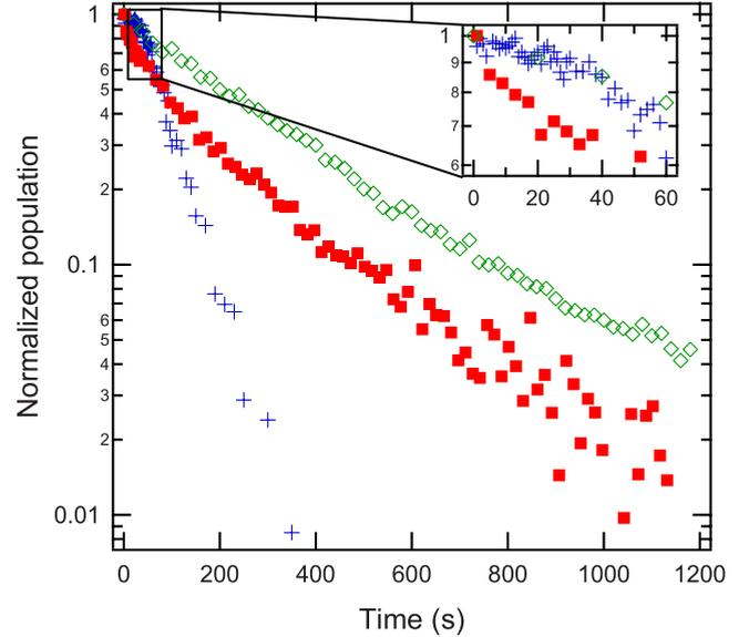
FIG. 7. (Color online) Number of atoms in the trap vs time, normalized to the initial loading for three difference cases: ( $\diamond$ ) pulse-cooled atoms, ( $\blacksquare$ ) continuously cooled atoms, and ( $+$ ) uncooled atoms. The inset shows the first 60 s of data.
