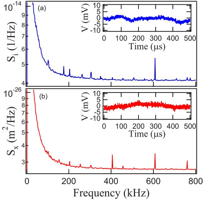
FIG. 4. (Color online) (a) Relative intensity noise power spectrum for the dipole trap laser, averaged over 50 runs. (b) Axial position noise power spectrum, averaged over 50 runs. Insets show the raw noise data for a typical run.
