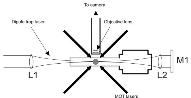
FIG. 1. Experimental setup. Rb atoms are trapped in a magneto-optical trap (MOT) and then transferred into an optical lattice.
