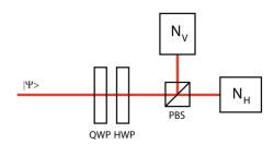
FIG. 1. (Color online) Apparatus for measuring the accessible density matrix for *N* photon polarizations. The state  $|\Psi\rangle$  is sent into a quarter wave plate (QWP) and half wave plate (HWP) followed by a polarizing beamsplitter (PBS). Number resolving photon counters count the number of vertical photons  $N_V$  and the number of horizontal photons  $N_H$ .
