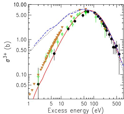
FIG. 4. (Color online) Triple-photoionization cross sections of Li. Black circles: This work. Green diamonds: Refs. [5,6]. Blue dashed line, calculated double-photoionization cross section of  $\text{Li}^+$  [13] (scaled); gray dotted line, measured double-photoionization cross section of He [3] (scaled); brown triangles, theory [20]; red solid line, shape function [23].
