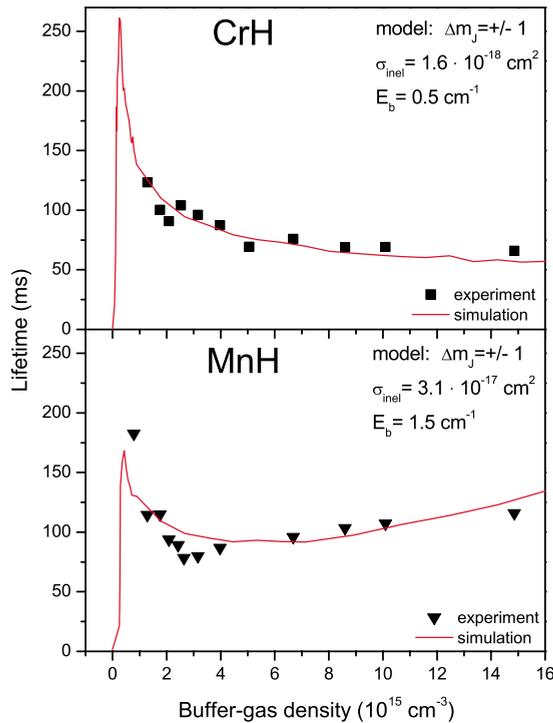
FIG. 7. (Color online) Calculated buffer-gas density dependence of the lifetimes of CrH and MnH molecules with inelastic-scattering cross sections of  $1.6 \times 10^{-18}$  and  $3.1 \times 10^{-17}$   $\text{cm}^2$ , respectively.
