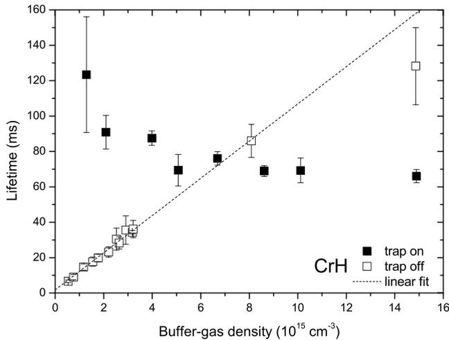
FIG. 3. Buffer-gas density dependence of the CrH lifetime in the presence (solid squares) and absence (open squares) of the magnetic trapping field. The dashed line is a linear fit of the field-free diffusion times excluding the point at the largest buffer-gas density.
