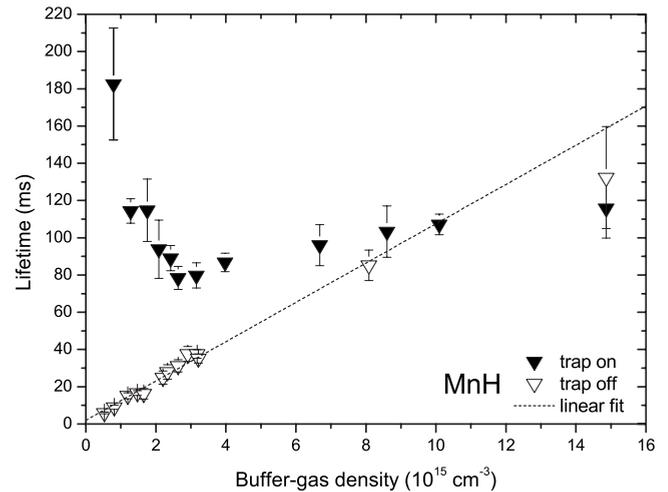
FIG. 4. Buffer-gas density dependence of the MnH lifetime in the presence (solid triangles) and absence (open triangles) of the magnetic trapping field. The dashed line is a linear fit of the field-free diffusion times excluding the point at the largest buffer-gas density.
