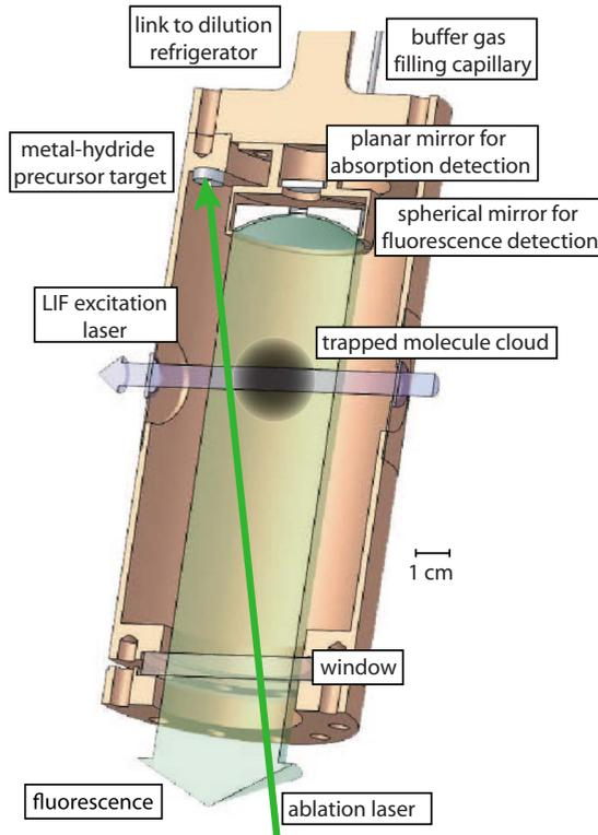
FIG. 1. (Color online) Scheme of the experimental setup, depicting a cut through the copper experimental cell. A hole in the spherical mirror to a planar mirror above allows for detection via absorption.
