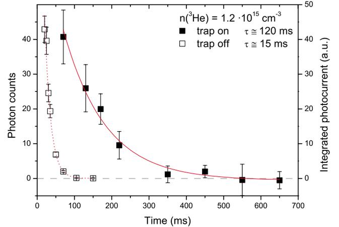
FIG. 2. (Color online) Time dependence of the fluorescence signal from CrH molecules after injection into the buffer-gas cell in the presence (solid squares: photon counts) and absence (open squares: integrated photocurrent) of the magnetic trapping field at a buffer-gas density of  $1.2 \times 10^{15} \text{ cm}^{-3}$ . Each data point represents the average of five measurements.
