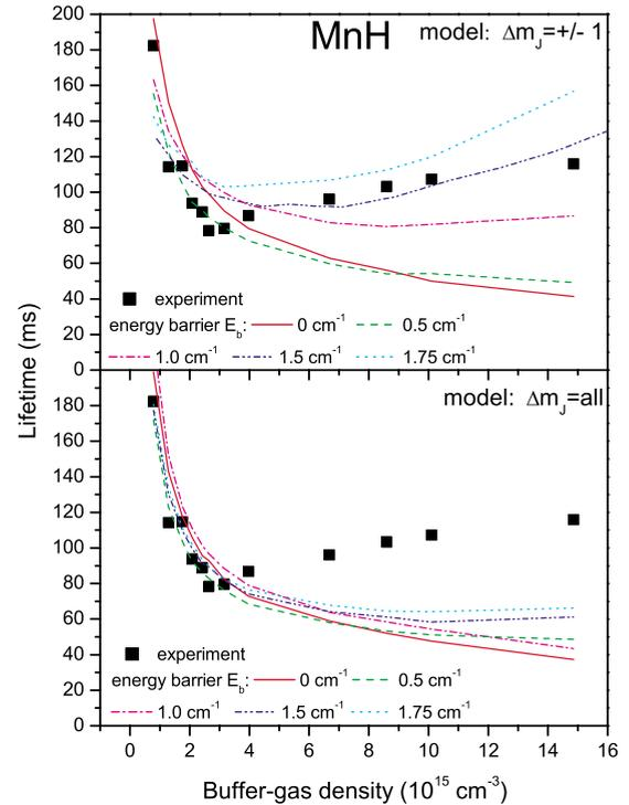
FIG. 6. (Color online) Simulated lifetime dependencies on the buffer-gas density of MnH, for two variants of the spin-flipping model. Each graph shows the best fit for selected inelastic collision energy barriers  $E_b$ . In the top curve, inelastic collisions are restricted to neighboring Zeeman states ( $\Delta m_J = \pm 1$ ); in the bottom graph, all energetically accessible Zeeman states are included. The experimentally obtained data are shown in both graphs as solid squares.
