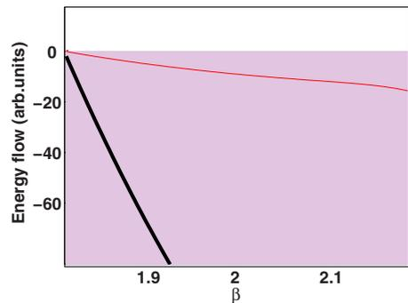
FIG. 7. (Color online) Total energy flow of the SWs in the first band gap vs  $\beta$  in the case of  $\alpha < 0$  for (a)  $\tilde{I}=0.01$  and (b)  $\tilde{I}=0.1$ . The other parameters are the same as Fig. 5.
