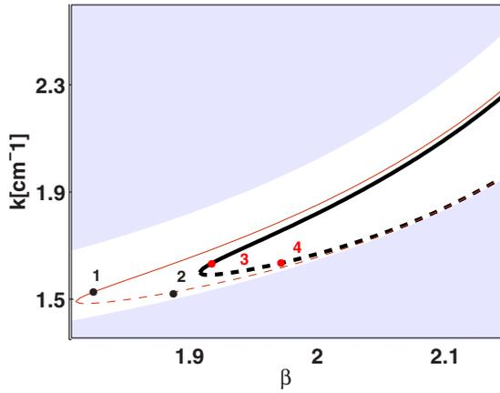
FIG. 2. (Color online) Dispersion property of the SWs in the first band gap for two different dimensionless intensity  $\tilde{I}=0.01$  (thin lines) and  $\tilde{I}=0.1$  (thick lines). Here unshaded regions show the first band gap of photonic crystal. The other parameters are the same as Fig. 1.
