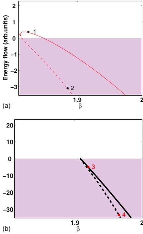
FIG. 4. (Color online) Total energy flow of the SWs in the first band gap vs  $\beta$  for one-humped (dashed line) and two-humped (solid line) structures in the case of  $\alpha > 0$  for (a)  $\tilde{I}=0.01$  and (b)  $\tilde{I}=0.1$ . The other parameters are the same as Fig. 1.
