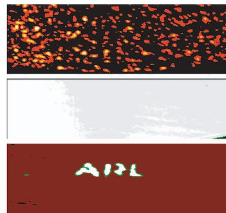
FIG. 3. (Color) Ghost image of “ARL” stencil. Upper: single frame CCD output. The “speckles” indicate typical random photo-detection events. This experiment does not have a point-to-point imaging relationship between the source and the CCD. Each speckle of the CCD can be excited by any or by all speckles of the source. Middle: time averaged CCD output of a few hundred frames. Lower: CCD- $D_1$  joint detection.
