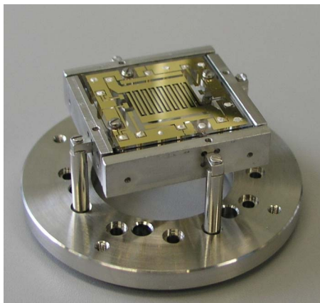
FIG. 3. (Color online) Photograph of one of the two ion trap chips mounted into its holder. The second chip (not shown) is mounted 5 mm above, facing the first chip. The metal bars surrounding the chip serve to shield the chip from electrostatic charging.
