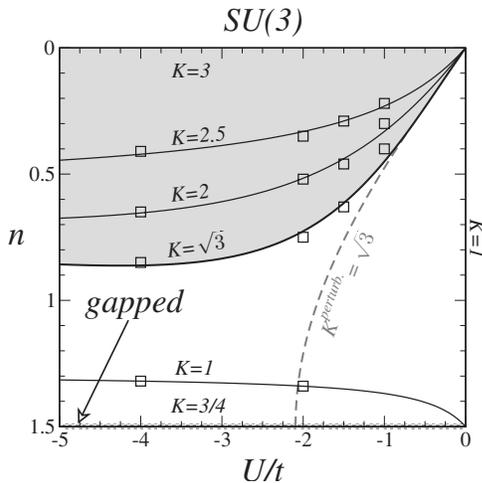
FIG. 3. SU(3) model. Phase diagram showing the Luttinger parameter  $K$  vs filling  $n$  and interaction  $U$ . The gray area is the superfluid triplet phase. Lines are guide for the eyes which behavior satisfies the perturbative limit close to the point  $(U/t=0, n=0)$ . We also plot the perturbative estimate separating both regions (see text), that agrees with our numerical finding at small  $|U|$  but deviates for large values.
