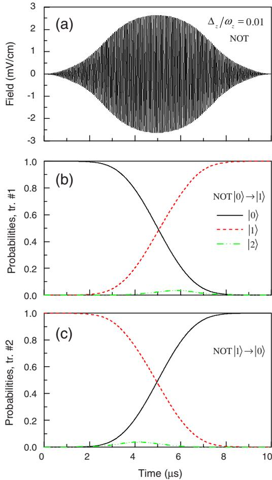
FIG. 1. (Color online) The gate NOT in the  $\text{Cd}^+$  ion trap with  $\omega_z/2\pi=2.77$  MHz and the anharmonicity parameter  $\Delta_z/2\pi=27.7$  kHz: (a) optimally shaped electric field; (b) switching of population between the qubit states during the NOT $|0\rangle\rightarrow|1\rangle$  transformation; (c) the same during the NOT $|1\rangle\rightarrow|0\rangle$  transformation.
