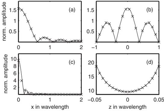
FIG. 2. Normalized time-reversed fields on the  $z$  axis (see Fig. 1 for details on the subplots). Here dipole transceivers time reverse the field. The  $\times$  marks are obtained by numerical integration of Eq. (10) and the continuous lines result from Eqs. (15) and (16).
