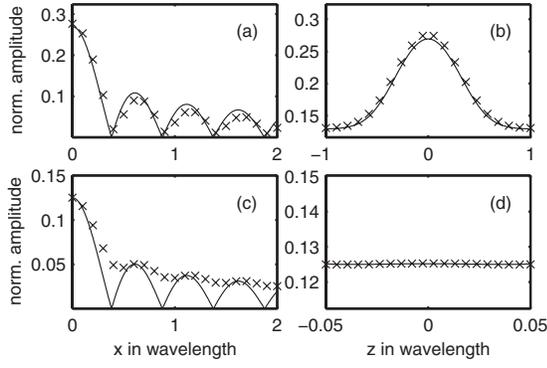
FIG. 3. Normalized time-reversed fields on the  $z$  axis (see Fig. 1 for details on the subplots). Here monopole transceivers time reverse the field. The  $\times$  marks are obtained by numerical integration of Eq. (10) and the continuous lines result from Eqs. (17) and (18). The plots are obtained with an attenuation length ( $1/\sqrt{\omega\epsilon}$ ) equal to a 126.2 wavelength.
