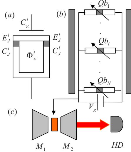
FIG. 1. (Color online) Scheme of our proposed experimental setups. (a) A qubit, (b) a series of qubits monitored by a unified gate voltage, (c) the total quantum device where the quantum network shown in (b) is loaded into the cavity formed by the reflective surfaces of mirrors ( $M_1, M_2$ ). The HD out of the cavity can allow the real-time determination of intracavity intensity  $I \propto |\langle a \rangle|^2$ .
