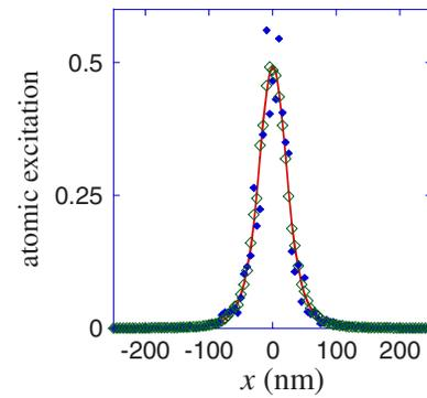
FIG. 4. (Color online) Numerical simulations that demonstrate the robust nature of our scheme. For the open squares, the intensity of the coupling laser beam fluctuates by  $\pm 10\%$  at each scanning point. For the solid squares, a timing jitter of  $\pm 0.01\ \mu\text{s}$  is assumed between the probe and coupling laser pulses. All the other parameters are identical to those of Fig. 3. The solid line is a replot of the numerical simulation of Fig. 3.
