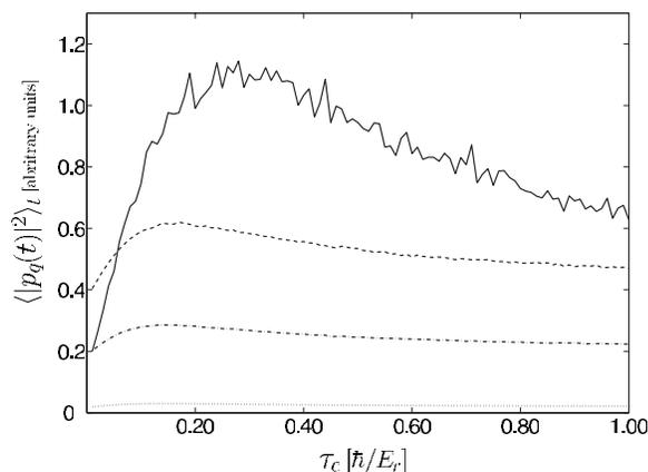
FIG. 6. Time-averaged population  $\langle |p_q(t)|^2 \rangle_t$  of the dipole (solid), quadrupole (dashed), octupole (dash-dot), and hexadecapole (dotted) modes as a function of the correlation time  $\tau_c$  of the RTN signal. The effective interaction was set to the value  $\tilde{g}=3.46E_r/q$ .
