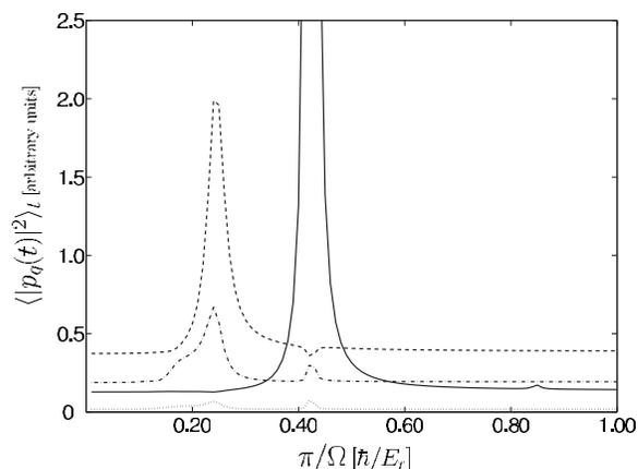
FIG. 7. Time-averaged populations  $\langle |p_q(t)|^2 \rangle_t$  of the dipole (solid), quadrupole (dashed), octupole (dash-dot), and hexadecapole (dotted) modes as functions of  $\pi/\Omega$ , where  $\Omega$  is the frequency of the harmonic drive. The effective interaction was set to the value  $\tilde{g}=3.46E_r/q$ .
