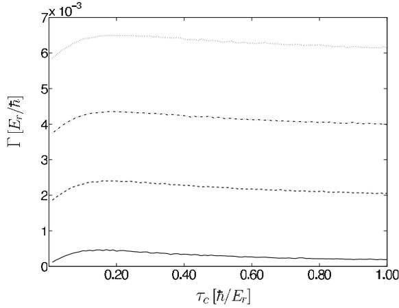
FIG. 4. Decay rate  $\Gamma$  as a function of the RTN correlation time  $\tau_c$  for four values of the effective interaction strength  $\tilde{g}/(E_r/q)=0, 6.91, 8.98, \text{ and } 10.4$ .
