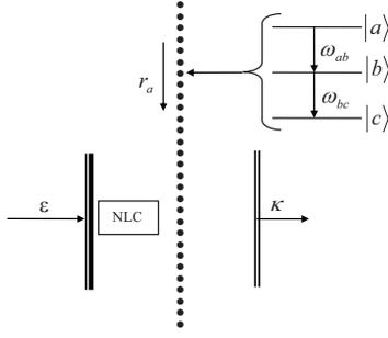
FIG. 1. Schematics of a nondegenerate three-level cascade laser with a subthreshold nondegenerate parametric oscillator.
