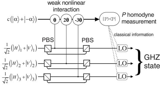
FIG. 1. Experimental scheme for generating the three-photon GHZ state. PBS represents polarization beam splitters and LO means local operation. For details, see text.
