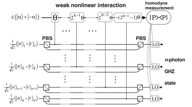
FIG. 4. Experimental scheme for generating the  $n$ -photon GHZ states.
